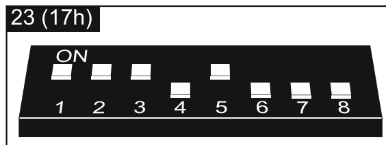
Fig. 21. Setting address in the INT-VG module / CA-64 SM expander. Recording of voice messages is disabled (switch 8 in OFF position).
